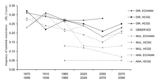
Fig. 6. Scenarios for the frequency of landslide reactivation ( $\phi$ ) obtained with different GCMs and downscaling methods. DIR = direct interpolation/transformation, MUL = multiple regression, ANA = analog-downscaling
