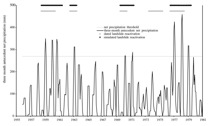
Fig. 2. Three-month sums of net precipitation compared to landslide reactivation, derived from tree ring analyses
