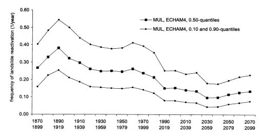
Fig. 7. Scenarios for the frequency of landslide reactivation ( $\phi$ ) obtained with multiple regression (MUL) and ECHAM4, showing 10, 50 and 90% quantiles of  $\phi$ . See text for explanation
